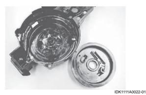
• Inspect the recoil rope. If the recoil rope is worn or damaged, replace it.
