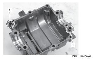
Install crankcase to cylinder. Apply engine oil lightly to 8 mm (0.31 in.) crankcase inside bolts only.
