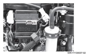
3) Remove the bolt and MAP sensor (1) from intake manifold.
