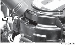
3) Check the ignition timing while operating the engine in neutral gear at 1 000 r/min.
