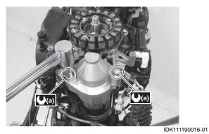
• Install flywheel and tighten flywheel nut to specified torque.
